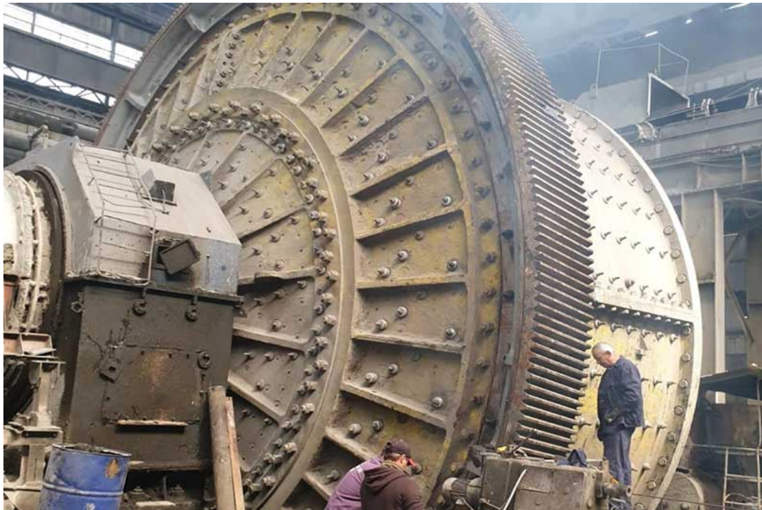
Commissioning Site of SAG Mill in Romania
