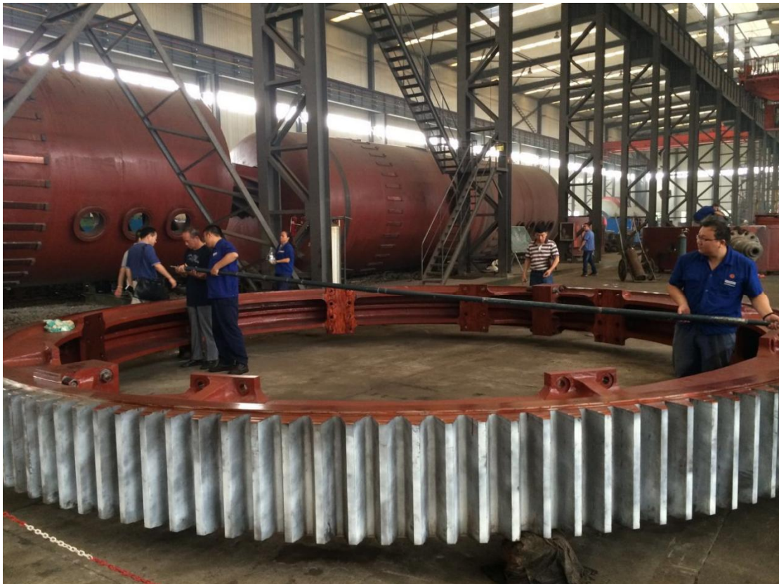
Inspection of Girth Gear for Turkish Customer
