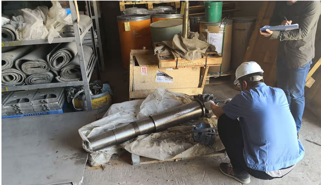
On-site Measurement of Pinion Shaft
