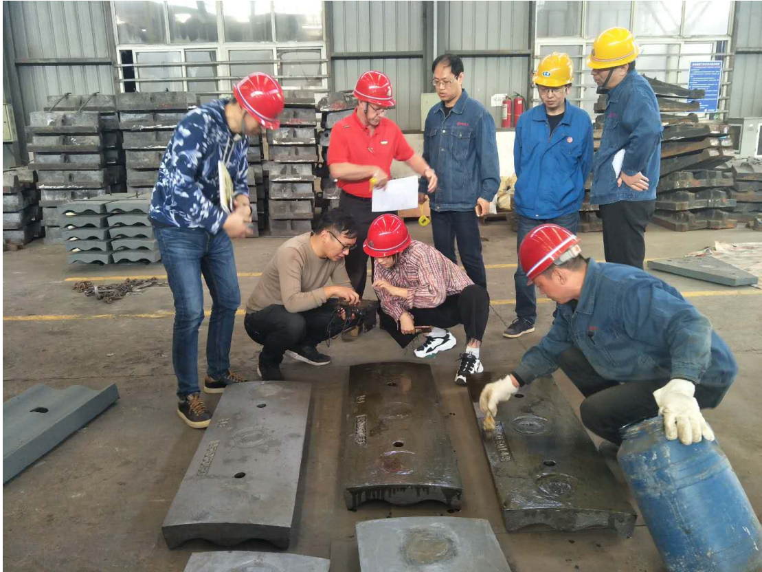
Inspection of ball mill liner for Australian FFF
