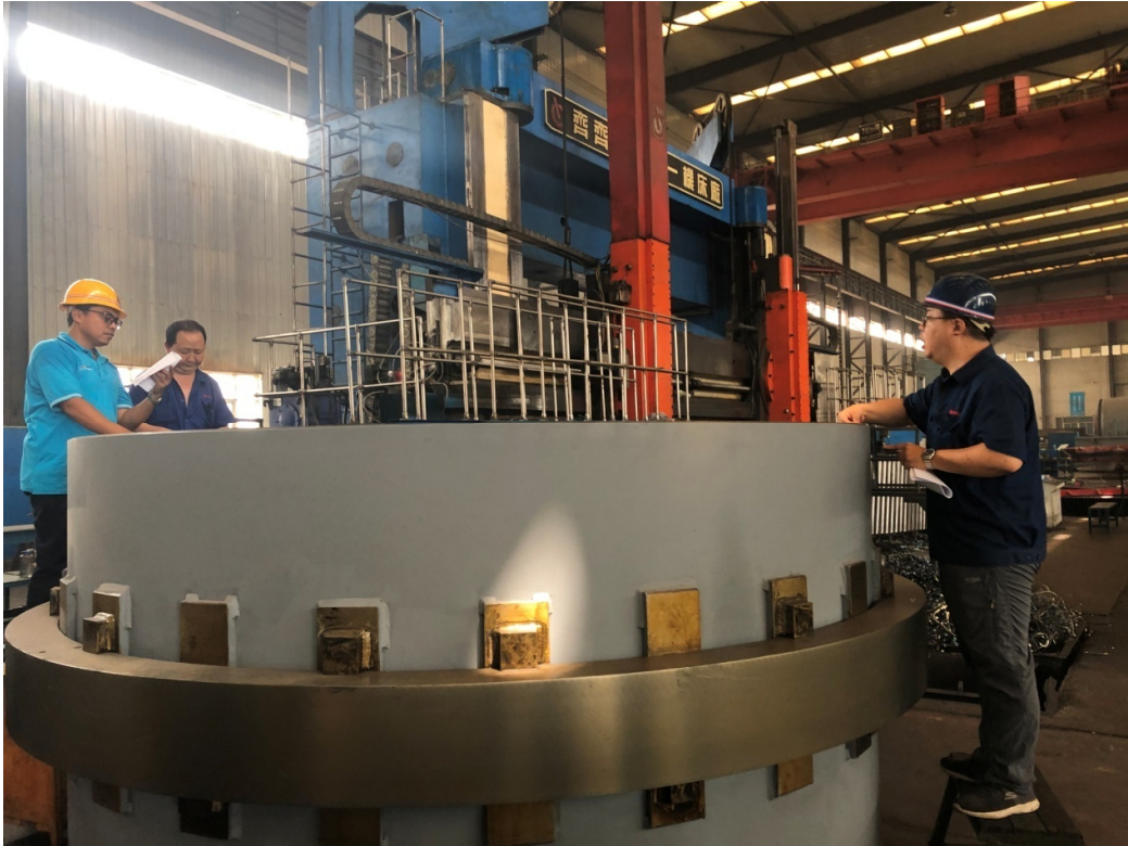
Inspection of Dryer Tyre for Indonesian Customers
