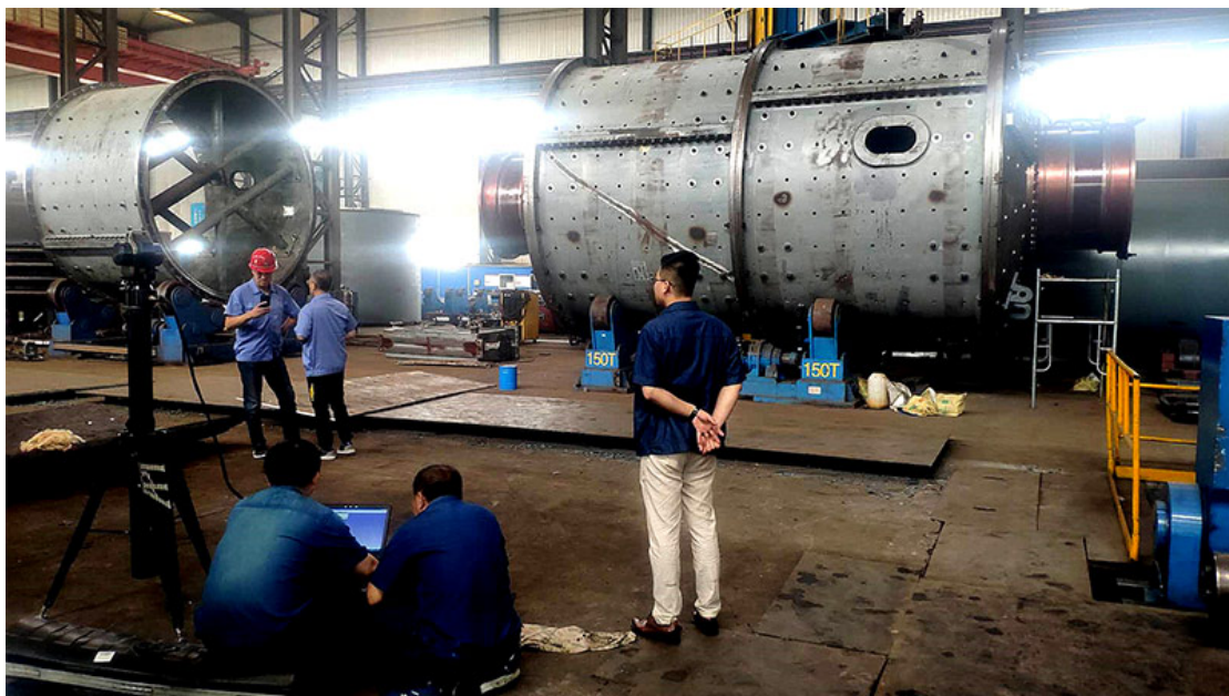
Coaxiality of the SAG Mill produced by CIC for Russian customers
