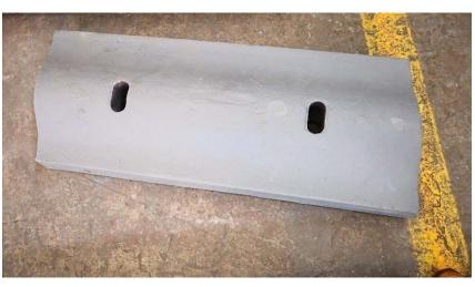
Φ3.2×11m Cement mill shell liner
