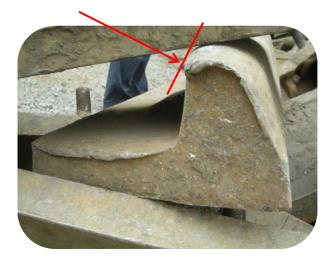
Poor Design :Liner Yield Deformation by Direct Smash of Balls Due
